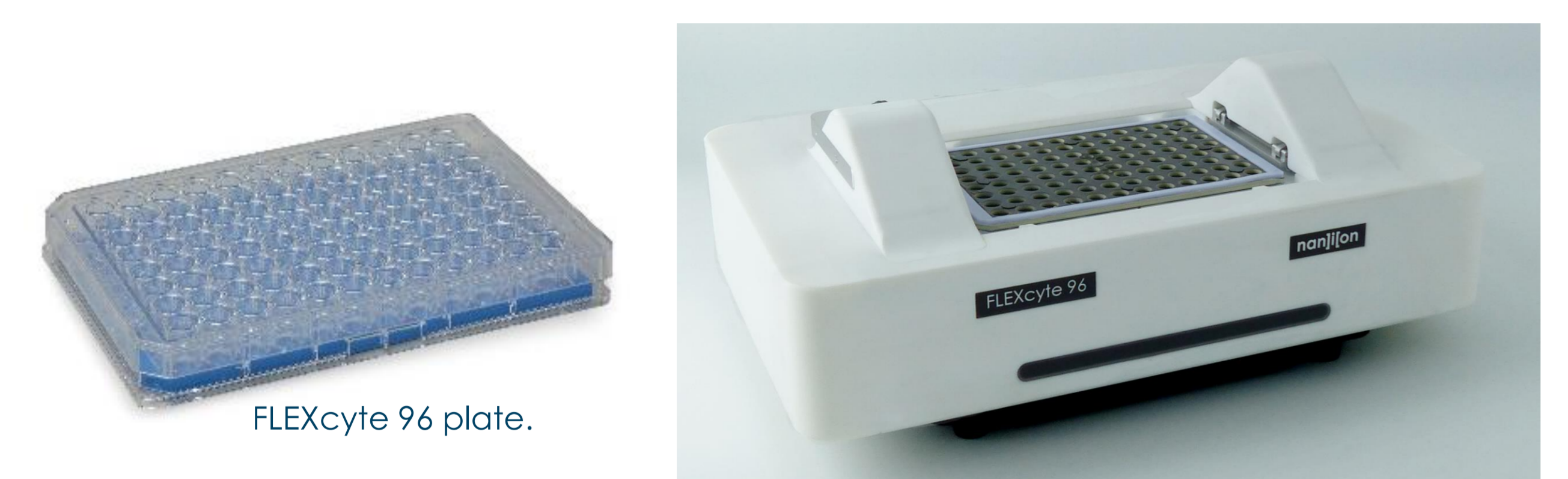
Picture of FLEXcyte 96 modified to have an active pressure regulation (a prototype). This system allows to apply a mechanical stress to the cell monolayer.
