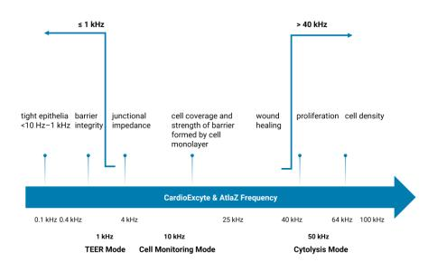
A frequency spectrum ranging from <10 Hz up to >64 kHz enables the analysis of a unique richness of cellular information, such as barrier integrity, cytolysis, cell monitoring or Transepithelial Electrical Resistance (TEER).
